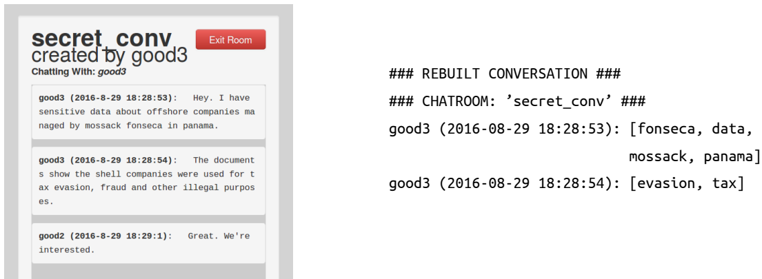
Figure 4.4: The conversation secret_conv seen by user good2 in the EncChat application, compared to the output of our attack program run by the adversary controlling the server and user bad .
